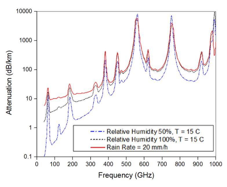
The attenuation peaks above 120GHz are due to water Above ~100GHz, the attenuation is too high for ground-based radio astronomy\* or for EESS to make measurements on the earth's surface.
