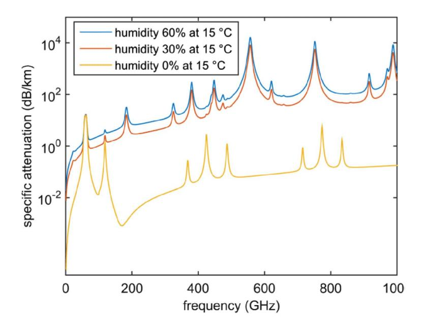
The attenuation peaks for 0% humidity – from atmospheric gases apart from water vapour – make no significant contribution to the total attenuation of moist air
