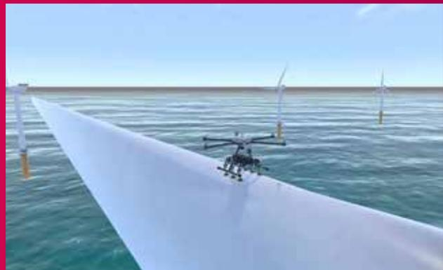
Figure 7: Deploying repair robot onto wind turbine
