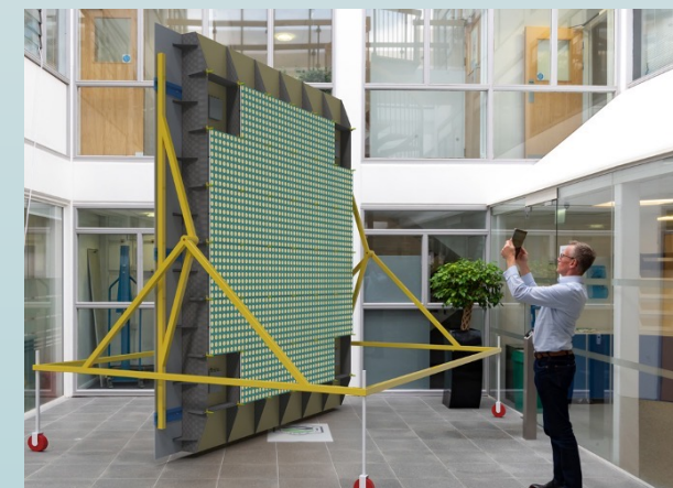
3m x 3m phased array antenna
